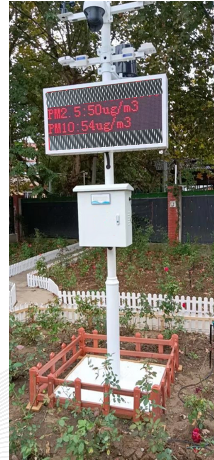
Automatic weather station
